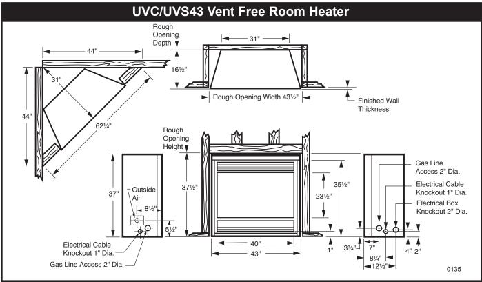
Fig. 2 UVC/UVS43 specifications and framing.
